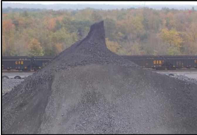
Moisture and freezing temperatures
